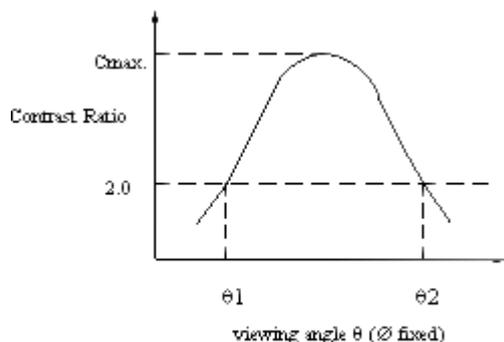
Remark: Optimum viewing angle with the naked eye and viewing angle  $\theta$  at  $C_{max}$
