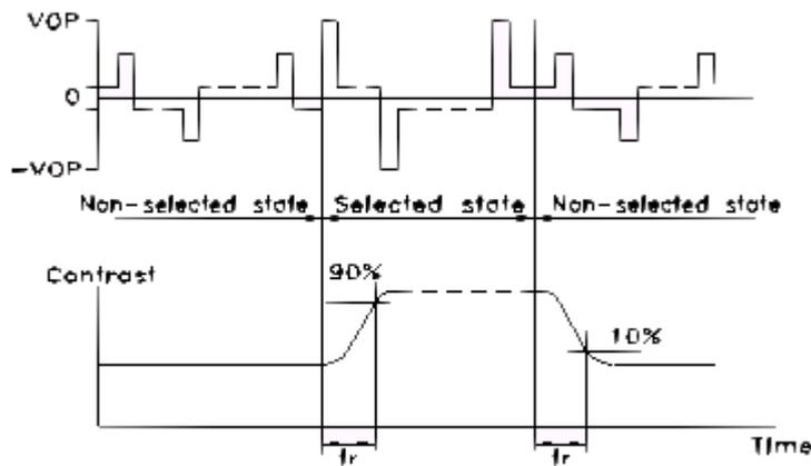
Note: Measured with a transmissive LCD panel which is displayed 1 cm<sup>2</sup>
