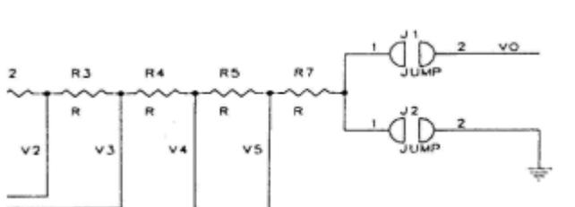
1. Internal: J2 short, add the appropriate resistor to R7 for contrast control.
