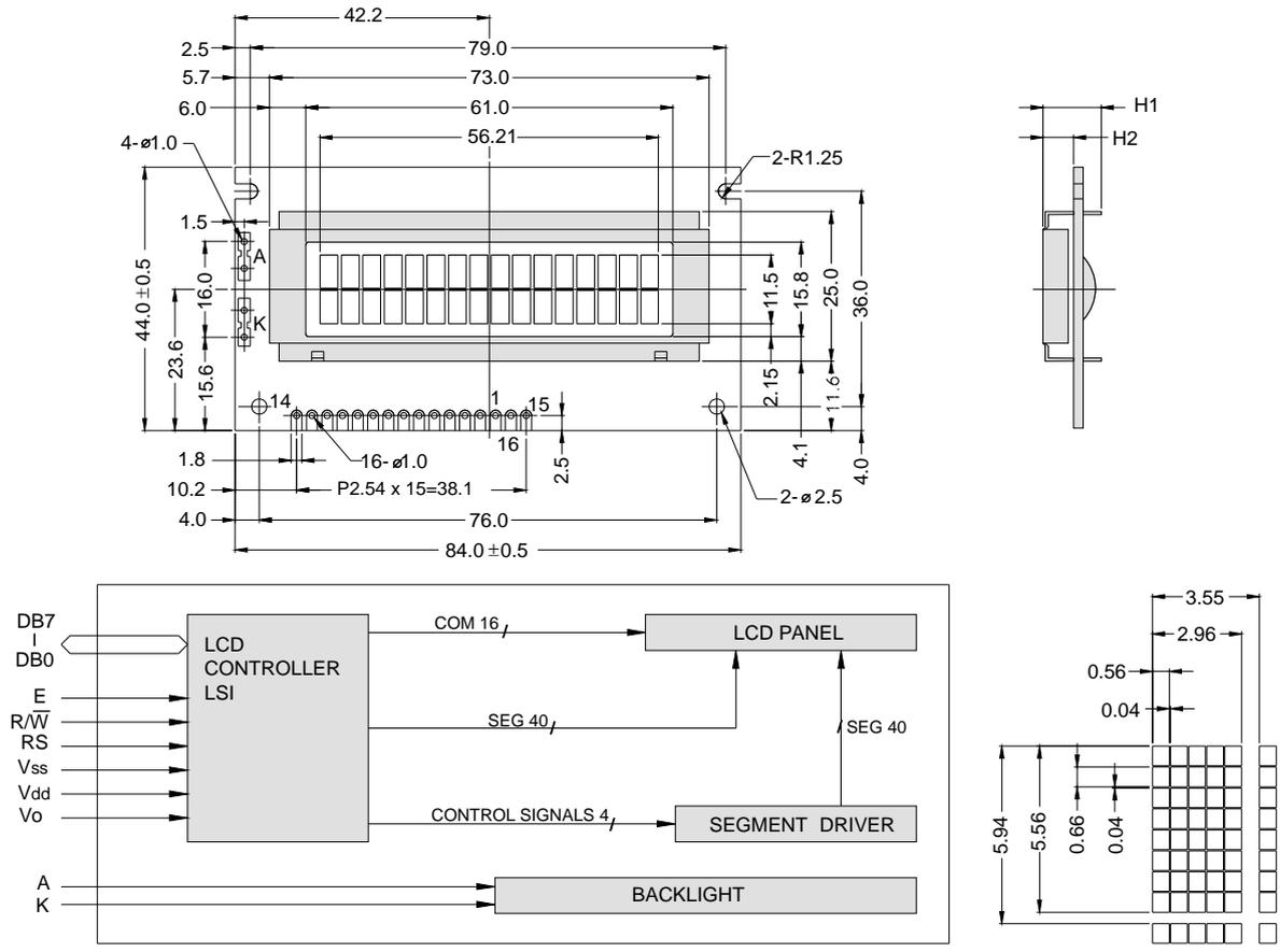
The tolerance unless classified  $\pm 0.3\text{mm}$
